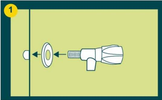
Unscrew the hose, and connect with the register, until adjustment (manual is sufficient)
